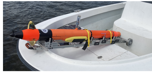
Fig. 6. Riptide Micro-UUV with modified payload
