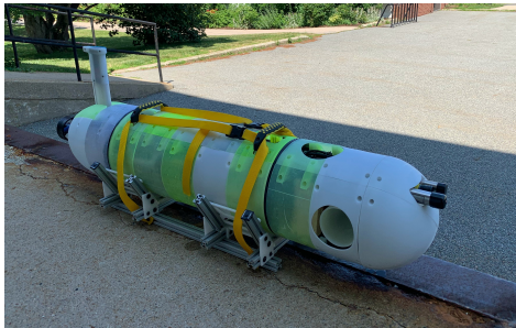
Fig. 4. ALPHA AUV at the loading dock of the Graduate School of Oceanography University of Rhode Island. The two tunnel thrusters can be seen on the nose and the main thruster on the stern side. The mast on the stern end of the vehicle is equipped WiFi, long range radio, and GPS.
